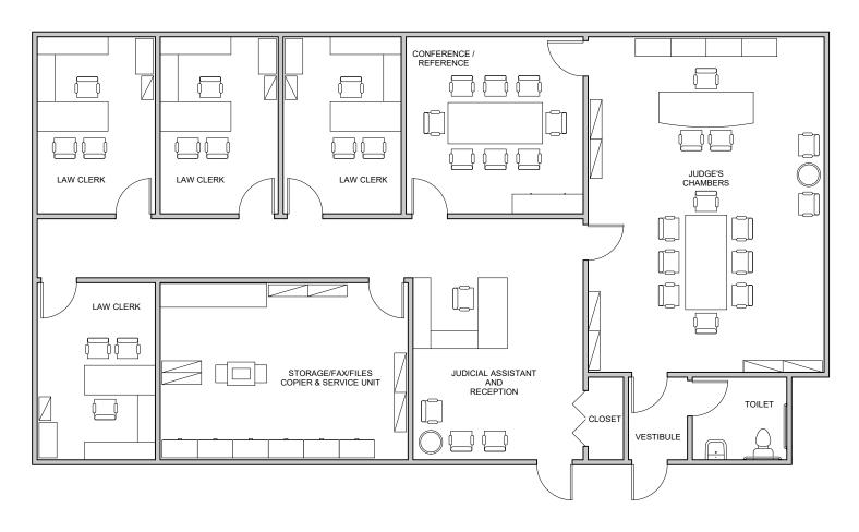
Note: The above figure illustrates a sample layout for a chamber suite. The actual design of chambers will vary according to the overall design of the courthouse. The sample has been provided to illustrate adjacencies and relative sizes of spaces.
