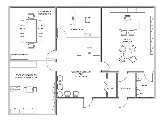
Note: The above figure illustrates a sample layout for a chambers suite. The actual design of chambers will vary according to the overall design of the courthouse. The sample has been provided to illustrate adjacencies and relative sizes of spaces.
