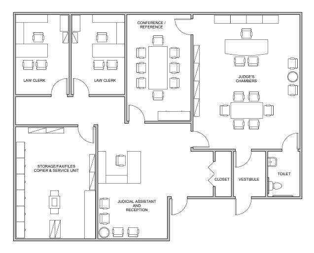
Note: The above figure illustrates a sample layout for a chambers suite. The actual design of chambers will vary according to the overall design of the courthouse. The sample has been provided to illustrate adjacencies and relative sizes of spaces.
