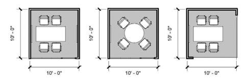
Note: Figure 18.14 demonstrates the benefits of modular design, using a 100 net SF enclosed room. Over time, the enclosed room can be adapted for various functions and uses without costly major renovations. Please refer to "Modularity" under the "Alternative Workplace Strategies Programming and Planning" section of this chapter for full description.
